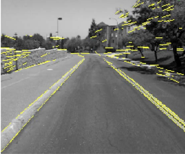
Figure 5. Driving video processed using Jean-Marc Pelletier's cv.jit.lines, a Max/MSP/Jitter tool for detecting line edges in video data.
