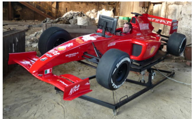
Figure 3. The F1Showcar, a full size motion simulator computer game car system.
