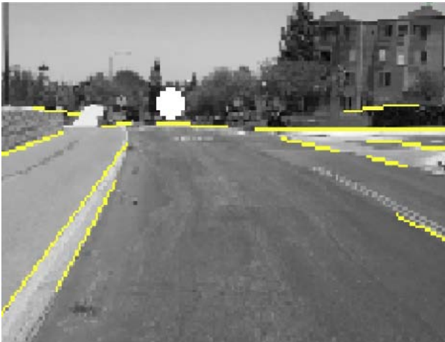
Figure 6. Driving video processed with cv.jit.lines and custom filtering modules. The dot in the center of the image shows the calculated direction of the road, which is the average convergence point of filtered lines.
